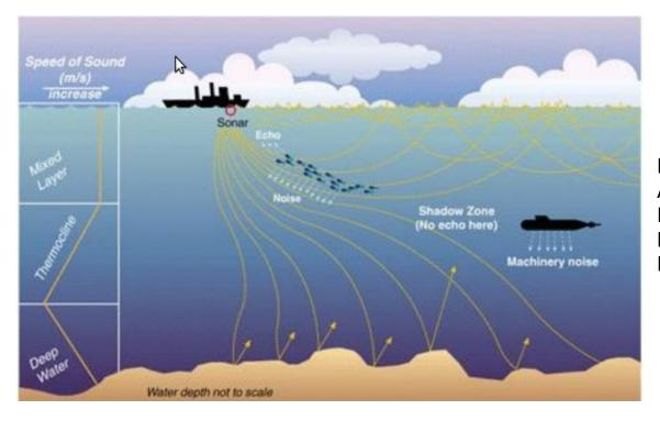
Propagation Delay (1500 m/s) Attenuation (depends on frequency) High Variablity (asymmetric links) Low Data Rate (1 kb/s) Noise
