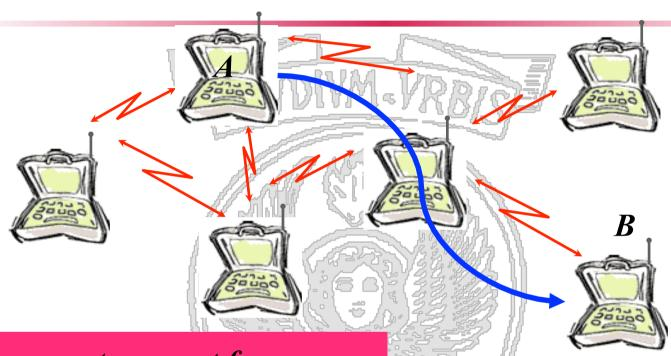
Routing must account for mobility, dynamicity (e.g., due to varying link quality and nodes alternating between ON and OFF states) and different resources available at the nodes
