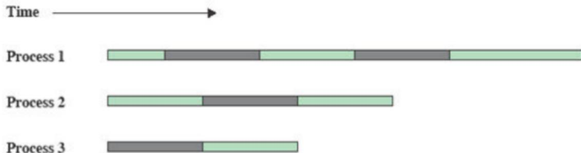
(b) Interleaving and overlapping (multiprocessing; two processors)
