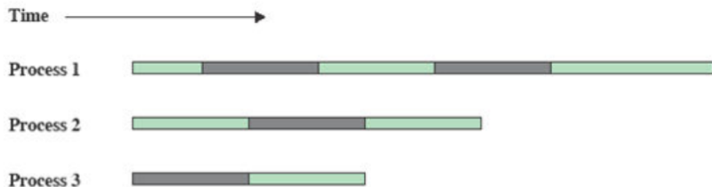
(b) Interleaving and overlapping (multiprocessing; two processors)
