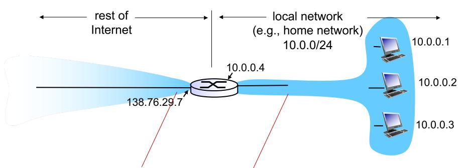
all datagrams leaving local network have same single source NAT IP address: 138.76.29.7,different source port numbers datagrams with source or destination in this network have 10.0.0/24 address for source, destination (as usual)
