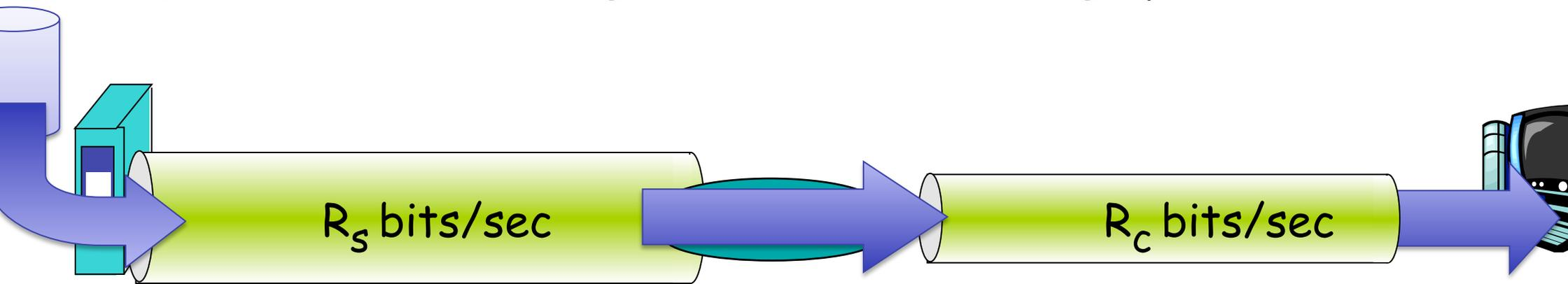
the bottleneck link on end-end path that constrains end-end throughput
