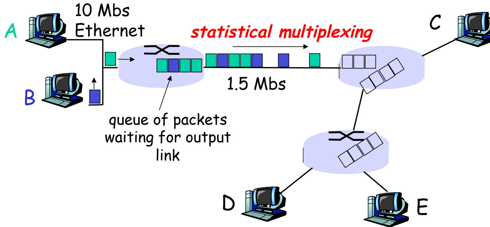
Sequence of A & B packets does not have fixed pattern ➡
