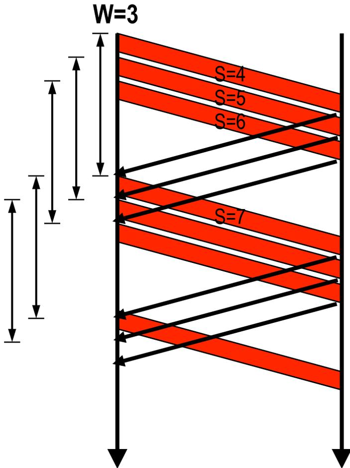
Dynamic window based reduces to pure sliding window when receiver app is very fast in reading data...
