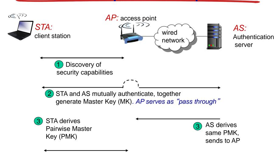
4 STA, AP use PMK to derive Temporal Key (TK) used for message encryption, integrity
