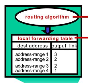
routing algorithm determines end-end-path through network
