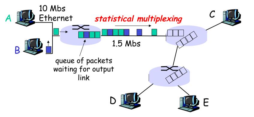
Sequence of A & B packets does not have fixed pattern **statistical multiplexing**.
