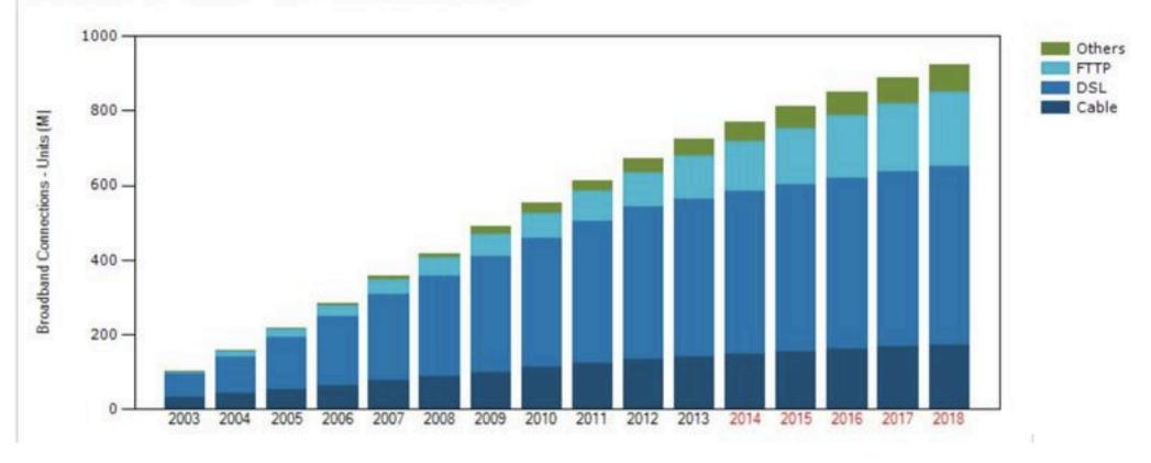
DSL is the most widely used broadband connection technology, and it's growing, but fiber-optic links are growing faster.
