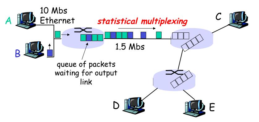
Sequence of A & B packets does not have fixed pattern **statistical multiplexing**.
