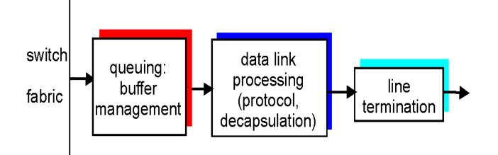
r *Buffering* required when datagrams arrive from fabric faster than the transmission rate
