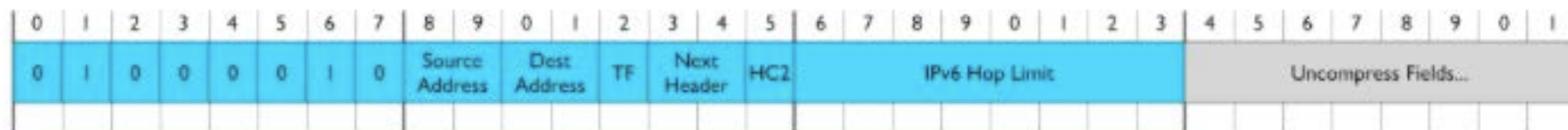
Figure 5. 6LoWPAN RFC 4944 IPv6 Header Compression.
