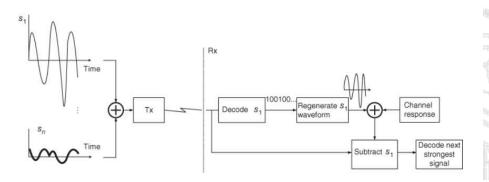
different users are superimposed into a single waveform. The receiver tries to decode the strongest signal while the other signals are treated as interference. The decoded signal is then regenerated into a waveform and subtracted from the composite received signal. The process is iterated for all desired signals. This method is called Successive Interference Cancellation (SIC), illustrated in Figure 13.2 for n user signals,  $s_1 \cdots s_n$ , where  $s_1$  is a strongest signal.
