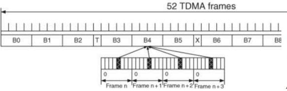
One radio block is allocated four slots in successive frames, that is, one block comprises  $4 \times 114 = 456$  bits, see Figure 4.8. Most of the slots in a Packet Traffic Channel (PTCH) are used for data transfer (PDTCH: Packet Data Traffic Channel) but a small fraction of the slots is used for signalling via a PACCH (Packet Associated Control Channel)
