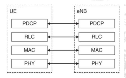
The scheduler is a part of the eNodeB MAC layer, it controls the assignment of uplink and downlink resources in terms of resource-block pairs in time and the frequency domain. The
