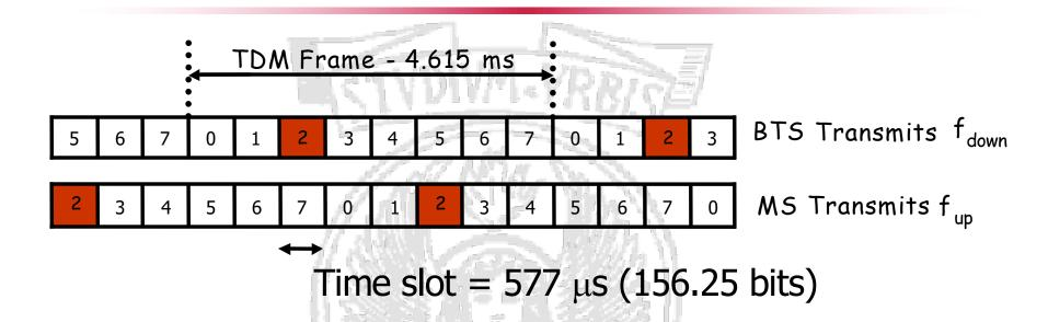
• On each radio carrier the TDMA structure allows us to create up to 8 channels for the transmission of voice encoded at 13 Kb/s
