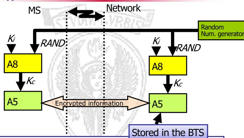
An additional level of security is provided by having the means to change the ciphering key, making the system more resistant to eavesdropping. The ciphering key may be changed at regular intervals as required by network design and security considerations.
