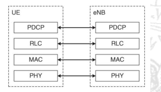
The scheduler is a part of the eNodeB MAC layer, it controls the assignment of uplink and downlink resources in terms of resource–block pairs in time and the frequency domain. The
