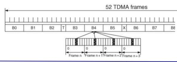
One radio block is allocated four slots in successive frames, that is, one block comprises  $4 \times 114 = 456$  bits, see Figure 4.8. Most of the slots in a Packet Traffic Channel (PTCH) are used for data transfer (PDTCH: Packet Data Traffic Channel) but a small fraction of the slots is used for signalling via a PACCH (Packet Associated Control Channel)
