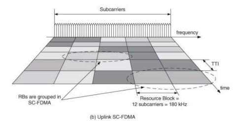
eNodeB in each TTI = 1 ms interval takes a scheduling decision and sends scheduling information to the selected set of terminals. The resource allocation is based on resource blocks (RBs), each consisting of 12 subcarriers occupying 180 kHz.
