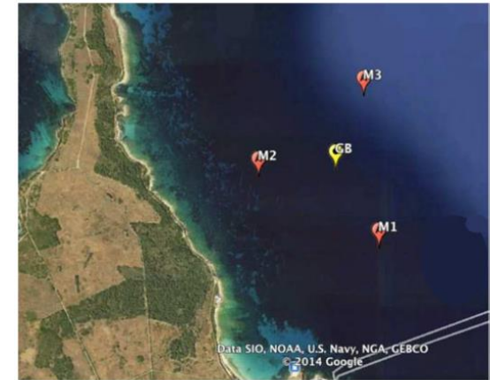
Fig. 1. Static node positions (red icons M1, M2, and M3) and gateway mooring (yellow icons GB).
