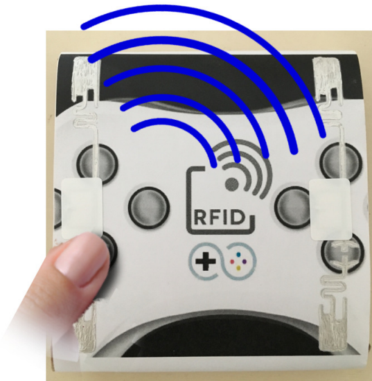
Figure 4: Button pressure on JoyPaper.
