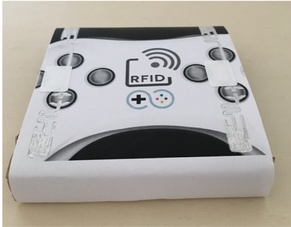
Figure 3: A JoyPaper featuring two buttons, realized through paper tags.
