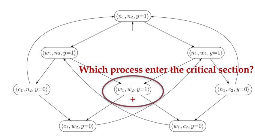
**Unfolding** of the program graph  $PG_1 \parallel PG_2$ : some states, e.g. $\langle c_1, c_2, y=0 \rangle$  are **not reachable**.
