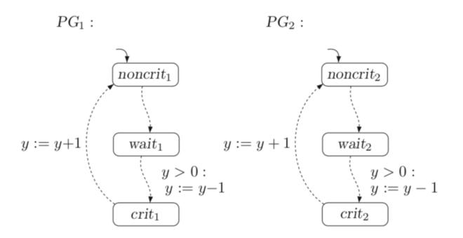
The **shared variable** *y* implements a **semaphore**, preventing both processes to enter the critical section simultaneously
