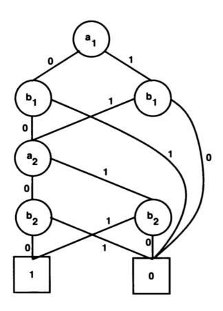
**Example**: two bit comparator:  $f(a_1, a_2, b_1, b_2) = a_1 \longleftrightarrow b_1 \land a_2 \longleftrightarrow b_2$
