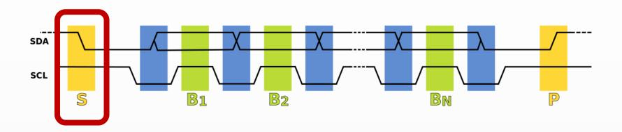
1. Data transfer is initiated with a *start* bit (S) signaled by SDA being pulled low while SCL stays high.
