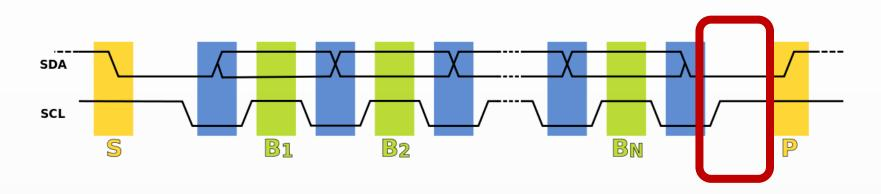
5. The final bit is followed by a clock pulse, during which SDA is pulled low in preparation for the stop bit.
