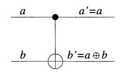
• The **second bit**, or target bit, is flipped if and only if the first bit is set to one and therefore  $b'=a \oplus b$
