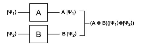
• The output after the inputs passed through gates A and B is:
