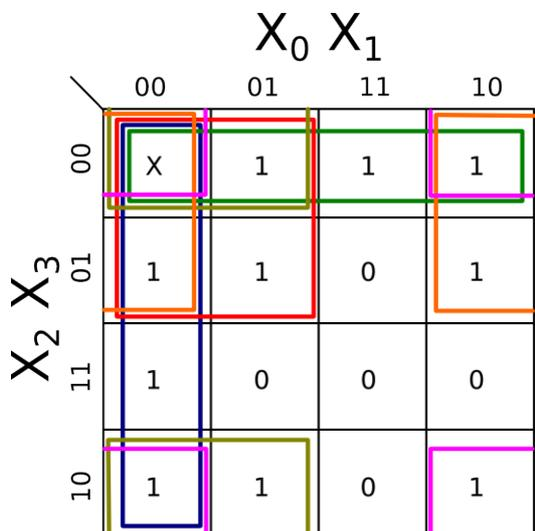
$$Y_1 = \overline{X_0}X_1 + X_2X_3 + X_1X_3 + X_0X_3 + X_1X_2 + X_0X_2$$
