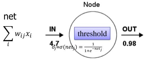
The activation function **limits** the node output values in [0 1] (threshold is 0 in the figure):
