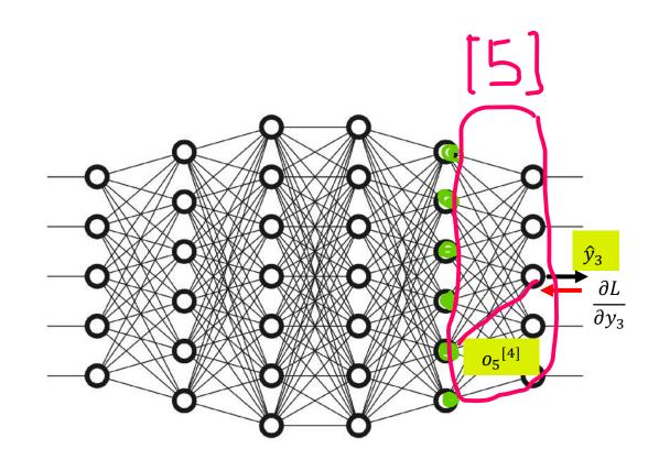
NOTE: COMMONLY, the quantity  $(y_j^h - \hat{y}_j^h)(1 - \hat{y}_j^h) \hat{y}_j^h$  is denoted with  $\delta_j^{[L]}$ , the contribution of output node  $n_j^{[L]} j$  to the total loss at step h. So we have  $\frac{\partial L}{\partial w^{[L]}_{ii}} = o_i^{[L-1]} \delta_j^{[L]}$
