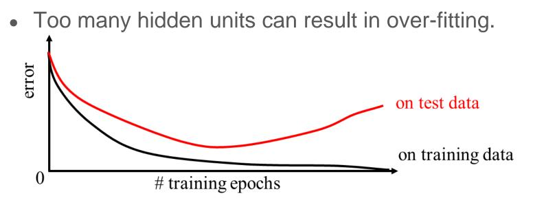
Use internal cross-validation to empirically determine an optimal number of hidden units (or use ML algorithms to learn the best architecture, <u>here</u> is an example).
