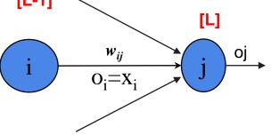
Note: for multiple layers, the input values  $x_i$  to node  $n_j$  in layer L is the output  $o_j$  of previous nodes in layer L-1, and  $w_{ij}$  is the synaptic weight of the connection  $i \rightarrow j$ .
