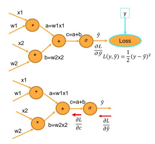
• Step 1 compute the partial derivative of the loss
