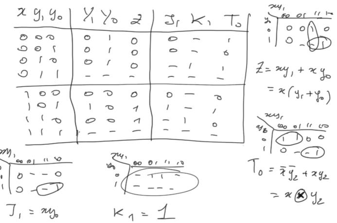
**Exercise 6 (4 points):** Design an automaton that receives in input two bit sequences and gives in output 1 whenever the last three bits of the first sequence followed by the last two bits of the second sequence represent a natural number in base 2 that is a multiple of 8. The first two outputs are ignored, hence you can handle them in the way that makes the automaton simpler.
