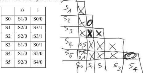
Minimize it and write down the associated sequential net that uses a JK FF for the most signifying bit and a T FF for the less signifying one.
