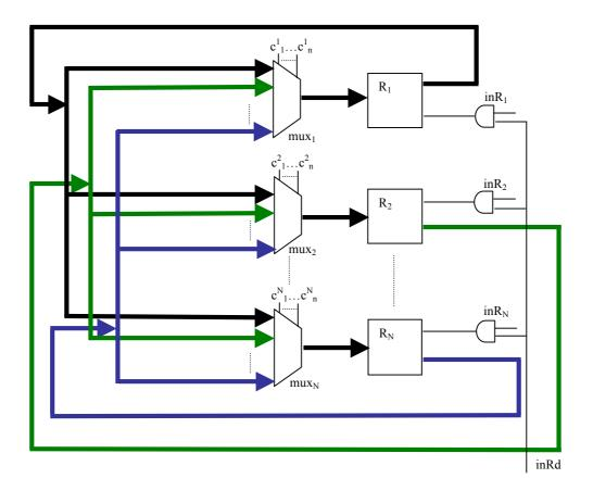
Again, the writing into a register is obtained through the AND between the global signal inRd and inR<sub>i</sub> (the writing signal for the specific register *i*). The selection of the source register for destination  $R_i$  is done through the control lines of mux<sub>i</sub>.
