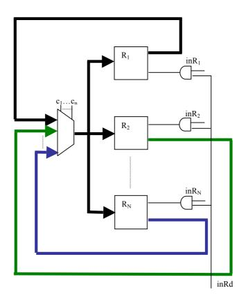
With this net, the content of  $R_i$  is output by the MUX if the control lines  $c_1...c_n$  provide the binary encoding of index *i*. The content of the source register is copied into the destination  $R_j$  whenever in $R_j$  and inRd both hold 1.
