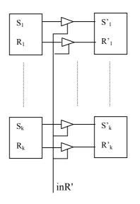
We can also design a net that allows for the bidirectional transfer of info between R and R'; in this case, we should also provide R with a control line inR:
