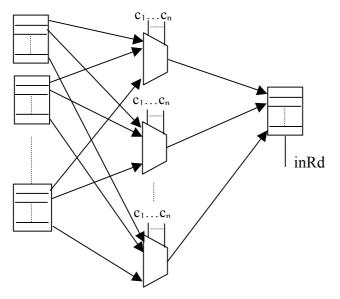
The first FF of every source register is connected with the first MUX, whose output goes to the first FF of Rd; the second FF of every source register is connected with the second MUX, whose output goes to the second FF of Rd; and so on until the last FF. The selection lines  $c_1, ..., c_n$ hold the same value for each MUX since they have to select one by one the bits of the same source register (the binary sequence  $c_1 c_2...c_n$  is the index i of the selected source register).
