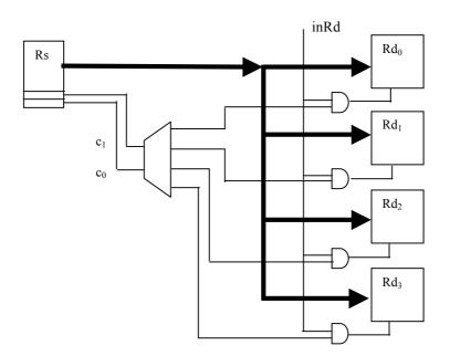
Notice that the control signals of the DEC are the two LSBs of the source register, as specified by the text.
