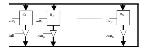
The interconnection is realized by using k lines (where k is the number of FFs of the registers): the *bus*. Registers' inputs directly come from the bus, whereas their outputs go into the bus by oassing through a (series of k) tri-state buffer. To copy the content of R<sub>i</sub> into R<sub>j</sub> we have to set line outR<sub>i</sub> of the *i*-th tri-state buffer and line inR<sub>j</sub> of the *j*-th register.
