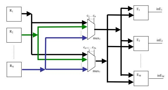
We have a (set of *k*) MUX for every operand in input to the computing modules: MUX1 selects the first operand among the *N* source registers through the control signals  $c_1...,c_n$ ; MUX2 selects the second operand through the control signals  $c_{n+1}...,c_{2n}$ , where, as usual, *n* is the upper integer part of  $\log_2 N$ . Every computing module has a control signal in  $E_j$  that enables reading and computing the operands previously stored in the input lines of module *j*.
