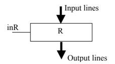
The thick arrow denotes a set of k lines, one for every elementary cell (FF) of the register; hence, we are auuming here a PIPO register. Line *inR* is used to simultaneously enable all the k elementary cells to writing.
