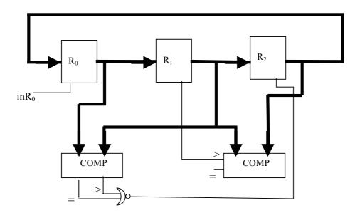
For in\_ $R_0$ , let us observe that the bitwise OR is simply performed as follows:
