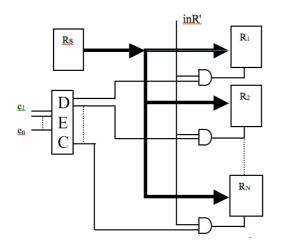
The control line in R' enables writing in one of the N destinations. The actual destination (that receives the content of register Rs) is register  $R_j$ , where j is binary encoded by the n selection lines  $c_1...c_n$ , inputs of the decoder; only the j-th output of the decoder is set.
