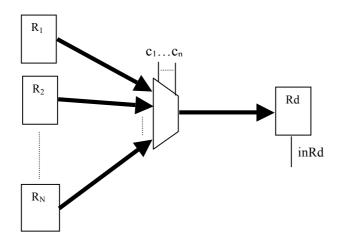
The control lines of the MUX  $c_1, ..., c_n$  (where n is the superior integer part of  $log_2 N$ ) provide the binary encoding of the index i of register  $R_i$  whose content must be copied into Rd. The above MUX, with thick inputs and output, actually denotes a set of *k* MUXs, one for each of the k FFs of the registers:
