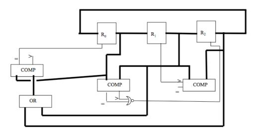
**Example 3 (A simplified ALU).** Design a many-to-many interconnection net that allows to move the content of two among N *k*-bits registers  $R_1...R_N$  to one between M computing modules (with two inputs)  $E_1....E_M$ .
