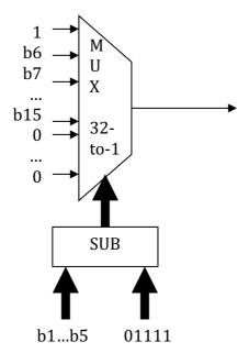
where here the thick lines represent numbers of 5 bits. This circuit gives in output 0 if and only if the integer part of the number stored in S0 is even, as desired.
