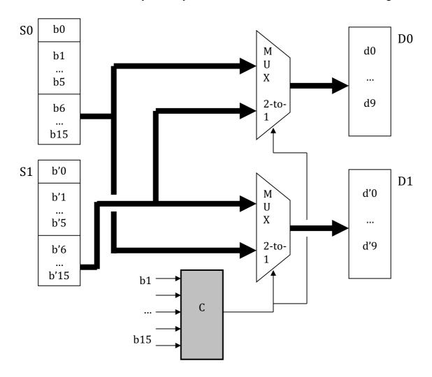
where the thick lines represent the 10 bits of the mantissas. As usual, the MUXs select the upper input if the control signal is 0, the lower input otherwise.
