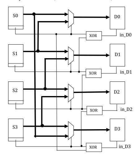
Without parallel transfers, we can use a bus. However, we must ensure the exclusive access to the bus, so we must select which transfer has to be performed (via 2 input signals, call them
