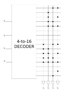
For the MUX, we use as control lines  $X_3$ ,  $X_2$  and  $X_1$ . Don't care symbols can be freely put to 0 or 1, but in our case it turns out that all 1s is a good option. So, the resulting circuit is:
