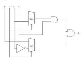
Exercise 1 (4+2 points): Analyze the circuit in figure (up to the minimal automaton). Then, provide the temporal diagram of the circuit with the input sequence 100110.
