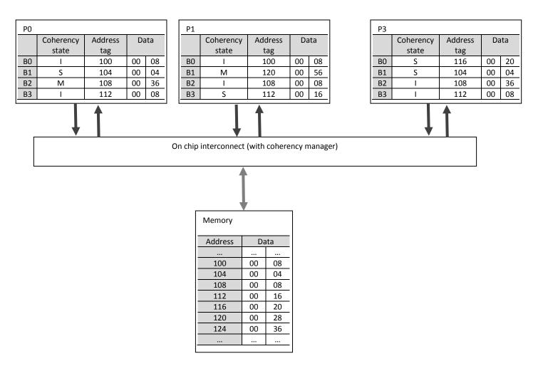
Each processor has a single, private cache with coherence maintained using the snooping coherence protocol. Each cache is direct-mapped, with four blocks each holding two words. The coherence states are denoted M, S, and I (Modified, Shared, and Invalid).
