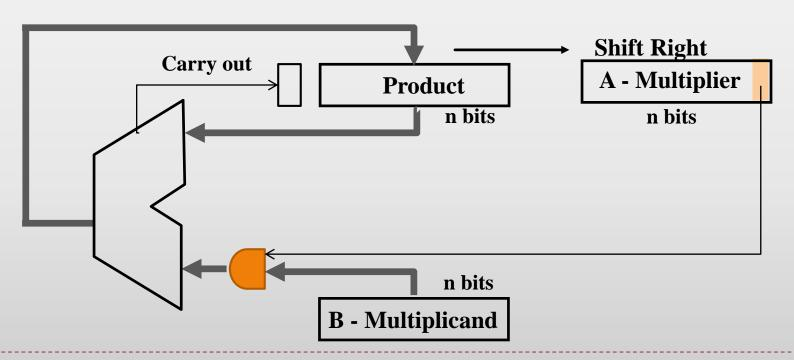
(ii) Registers P and A are shifted right, with the carry-out of the sum being moved into the high-order bit of P, the low-order bit of P being moved into register A, and the rightmost bit of A (not used in the rest of the algorithm) being shifted out
