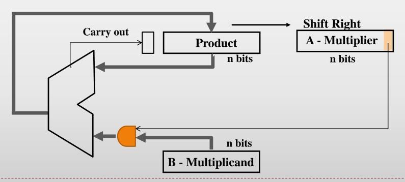
Then, we replace a string of 1s in multiplier with an initial subtract when we first see a one and then later add for the bit after the last one
