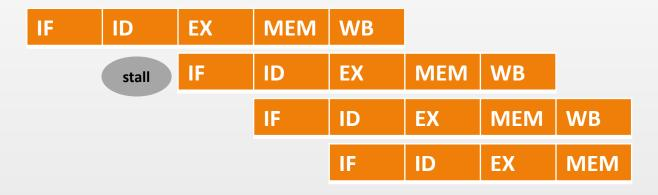
► Each branch costs **one stalls** to fetch the correct instruction flow: (PC+4) or Branch Target Address
