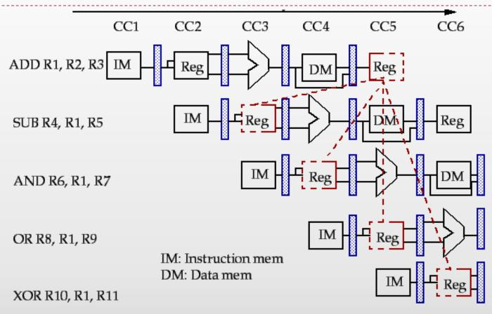
The XOR instruction operates properly because its register read occurs in clock cycle 6, after the register write
