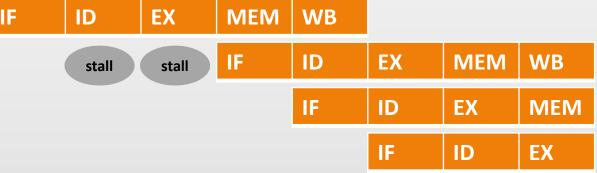
Each branch costs two stalls to fetch the correct instruction flow: (PC+4) or Branch Target Address
