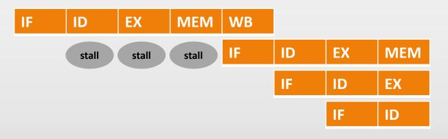
▶ Each branch costs three stalls to fetch the correct instruction flow: (PC+4) or Branch Target Address
