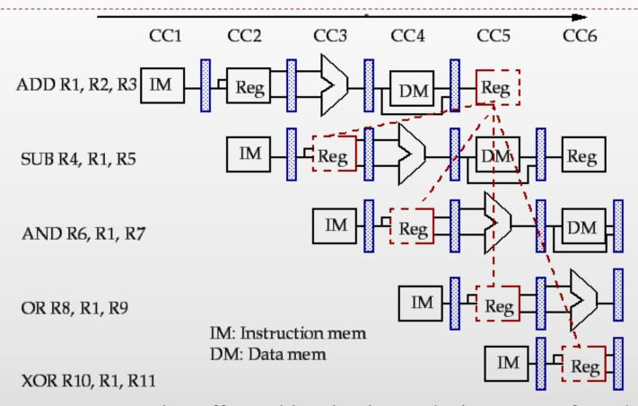
AND instruction is also affected by this hazard: the write of R1 does not complete until the end of clock cycle  $5 \rightarrow$  the AND instruction that reads the registers during clock cycle 4 will receive the wrong results
