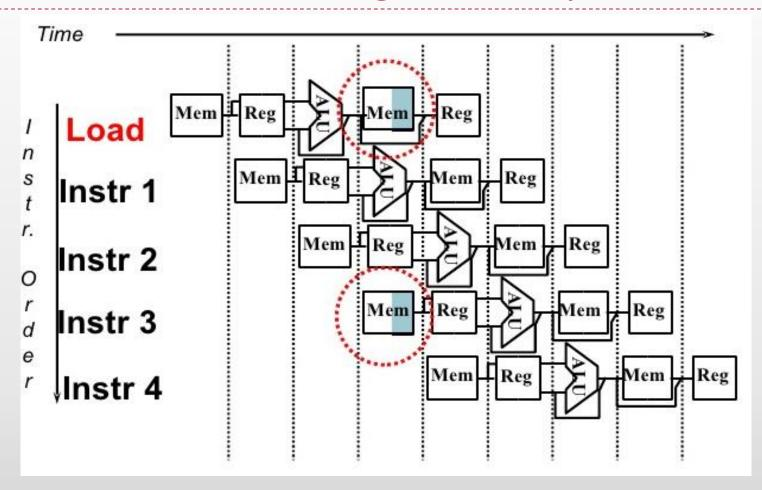
To resolve this hazard, we **stall** the pipeline for **1 clock cycle** when the data memory access occurs
