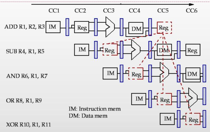
The OR instruction also operates without incurring a hazard because we perform the register file reads in the second half of the cycle and the writes in the first half
