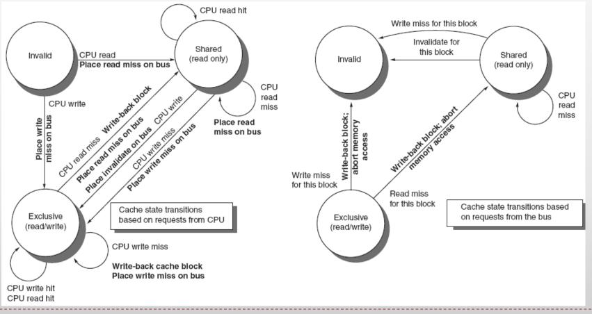
There is only one finite-state machine per cache, with stimuli coming either from the attached processor or from the bus
