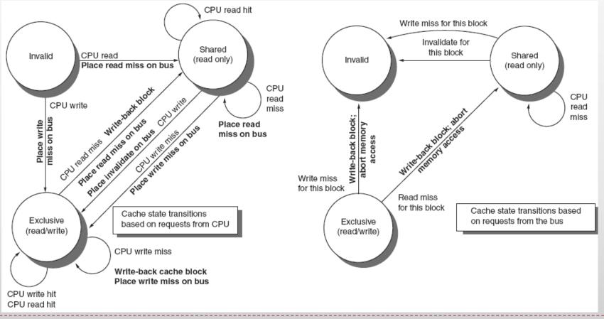
The three states of the protocol are duplicated to represent transitions based on processor requests (left), and bus requests (right)
