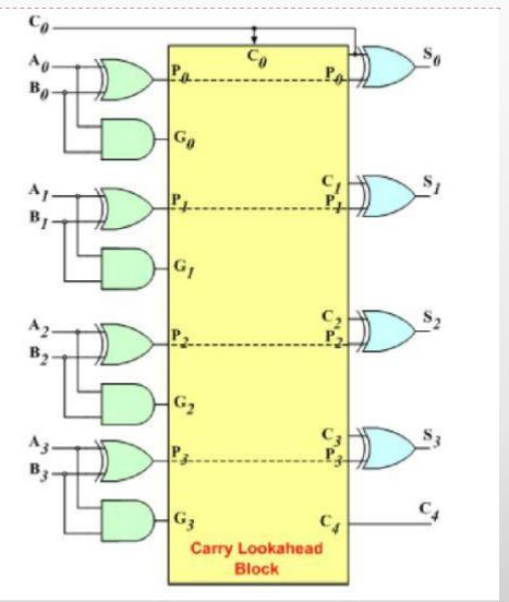
If we consider 4 bits, we have that  $c_1$ ,  $c_2$ ,  $c_3$ ,  $c_4$ , depend only on  $c_0$ :
