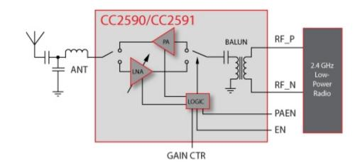
Interchangeable 2.4GHz ISM band Front-ends:
