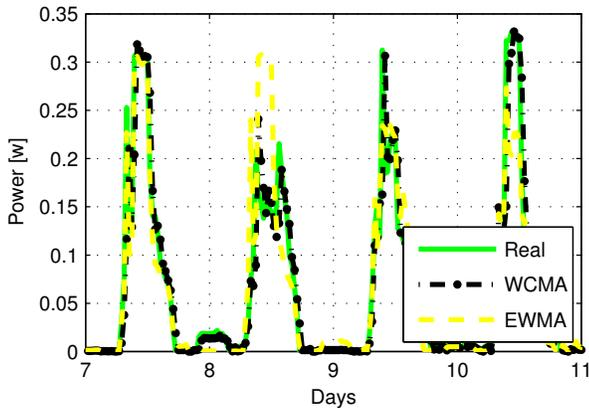
Fig. 4. Prediction accuracy of WCMA vs. EWMA
