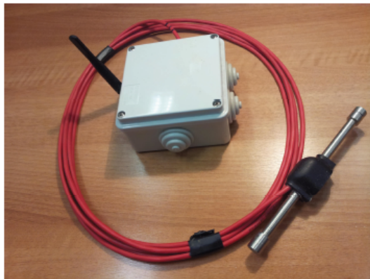
SISGEO OVK4200VC00 Dedicated interface board for TelosB mote Energy consumption: 720 mJ
