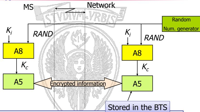
An additional level of security is provided by having the means to change the ciphering key, making the system more resistant to eavesdropping. The ciphering key may be changed
