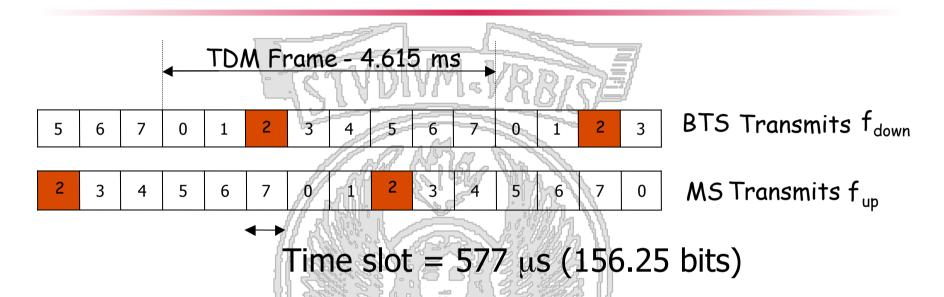
• On each radio carrier the TDMA structure allows us to create up to 8 channels for the transmission of voice encoded at 13 Kb/s
