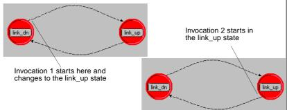
When a process model enters a state, it executes the enter executives and then, if the state is unforced (as above), the process model stops execution and returns control to the simulation. We'll discuss forced and unforced states in more detail later.
