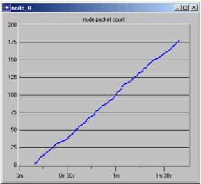
As illustrated in this graph, the results of the simulation indicate that the total number of packets received steadily increases over the simulation duration, though not at a perfectly constant rate. As expected, with two sources delivering packets each at a mean of 1 packet/second, the total number of packets received after 90 seconds of packet generation (packet generation commences after 10s of simulation time) is about 180.
