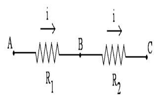
$$V_A - V_C = (V_A - V_B) + (V_B - V_C) = i R_1 + i R_2 = i(R_1 + R_2)$$
