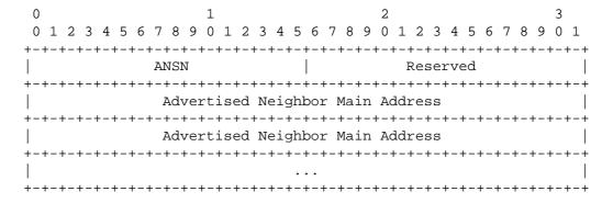
This is sent as the data-portion of the general message format with the "Message Type" set to TC\_MESSAGE. The time to live SHOULD be set to 255 (maximum value) to diffuse the message into the entire network and Vtime set accordingly to the value of TOP\_HOLD\_TIME, as specified in section 18.3.
