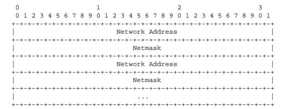
This is sent as the data part of the general packet format with the "Message Type" set to HNA\_MESSAGE, the TTL field set to 255 and Vtime set accordingly to the value of HNA\_HOLD\_TIME, as specified in section 18.3.
