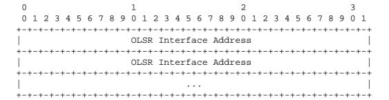
This is sent as the data-portion of the general packet format described in section 3.4, with the "Message Type" set to MID\_MESSAGE. The time to live SHOULD be set to 255 (maximum value) to diffuse the message into the entire network and Vtime set accordingly to the value of MID\_HOLD\_TIME, as specified in section 18.3.
