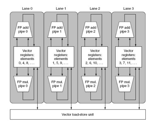
Figure illustrates how to improve vector performance by using parallel pipelines to execute a vector add instruction
