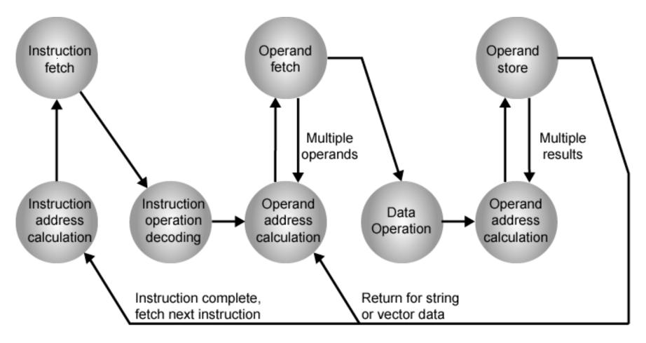
**Instruction operation decoding** (iod): Analyze instruction to determine type of operation to be performed and operand(s) to be used
