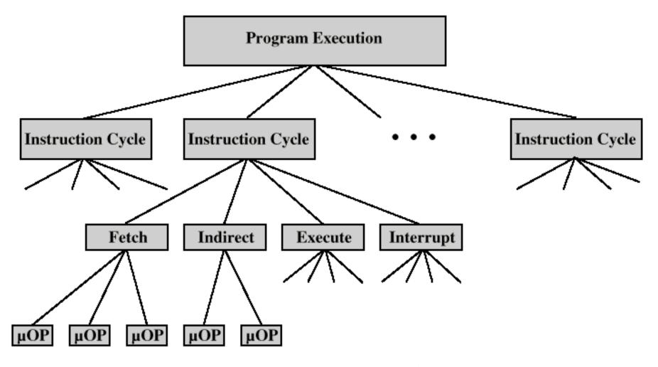
The instruction cycle is decomposed into sequence of elementary *micro-operations*
