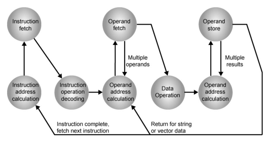
Operand address calculation (oac): If the operation involves reference to an operand in memory or available via I/O, then determine the address of the operand
