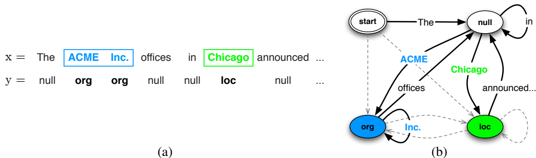
Figure 7: An information extraction example viewed as a sequence labeling task. (a) A sample input sequence x and corresponding label sequence y . (b) A sequence model represented as a finite state machine, illustrating the path of \langle x, y \rangle through the model.
